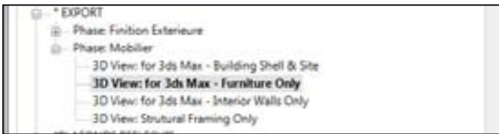
Views with the same parameter “*Export” grouped together the Revit project browser
