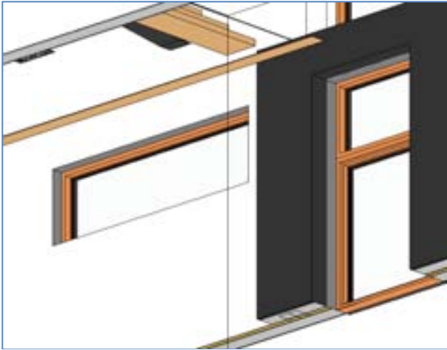
Edges/Borders around windows are assigned to a default material.
